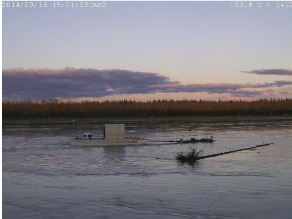
Figure 6. Test barge with an Oceana Energy, Inc. turbine on deck behind the instrument tent, tethered behind the RDDP at the Tanana River Test Site, Alaska. A large debris object floats downstream nearby. (Photo taken by the Video Debris Observation System)
