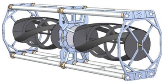
**Fig. 4** Example of a crossflow turbine with the axis orthogonal to the river current as in this design proposed for the Nenana, Alaska hydrokinetic project (image courtesy of Ocean Renewable Power Company)
