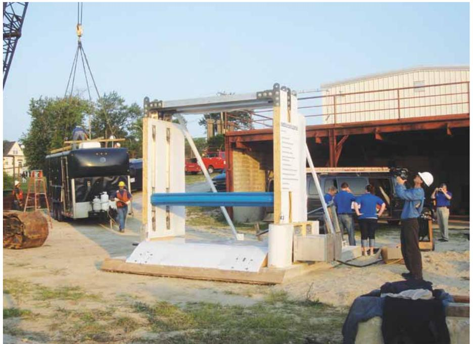
The Vortex Hydro VIVACE hydrokinetic power conversion device that operates from the principal of vortex induced shedding induced oscillations.
