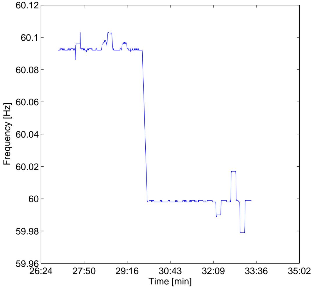
Figure 3.2: Frequency response during transition to diesel-off mode. The transition occurs at 30 min and the GRIDFORM inverter is able to hold frequency very close to the nominal 60 Hz. The deviations in diesel-off mode are due to load changes. Data shown was taken with the Fluke<sup>®</sup> 435 Series II Power Quality and Energy Analyzer at the load bank transformer.
