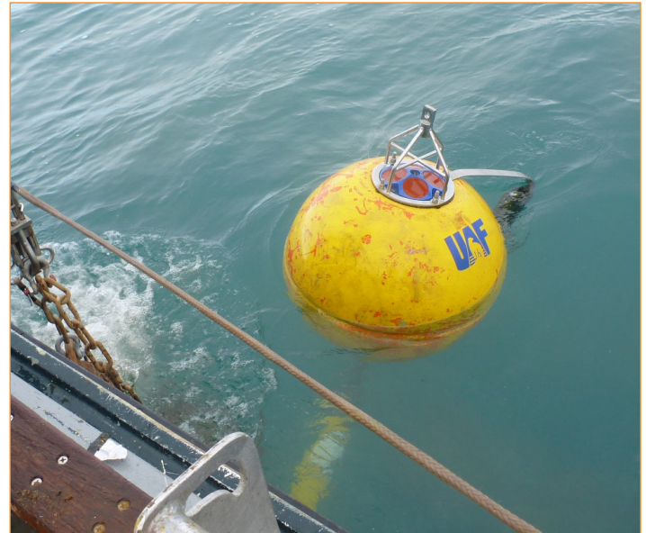
Mooring top float with ADCP visible in the center of the float. The float is tethered to an 800-pound weight (a train wheel) that sits on the seafloor. A small "acoustic release" (the yellow cylinder to the right of the float) between the float and the weight allows for the retrieval of the float when the mooring is recovered for data download. The train wheel remains on the seafloor. This arrangement allows the sensitive instrumentation to remain far removed from the surface where large breaking waves could cause damage and at the same time keeps the instruments above the seafloor, where constantly moving waves of sand would likely bury anything located there. Photo courtesy of J. Kasper, UAF
