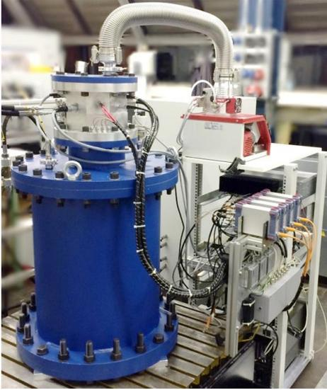
**Figure 3: Photo of the outer-rotor prototype**
