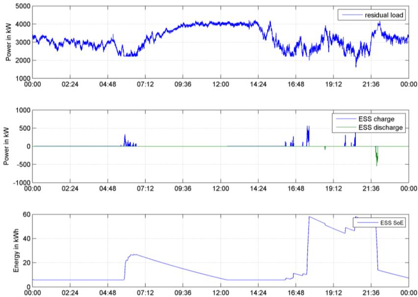
**Figure 8: Simulated power and capacity profile of the KESS in operation (day 10/14)**
