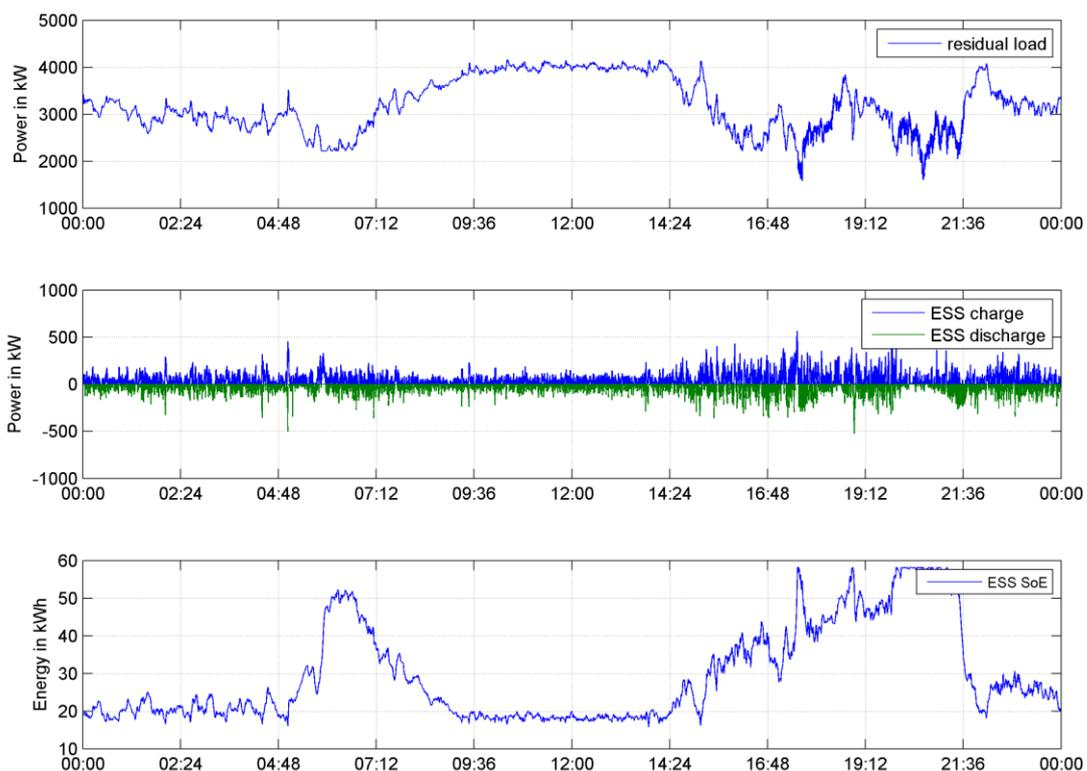
**Figure 10: Storage profile for the first day of the second week with combined application load smoothing and providing SRC (day 10/14), compare Figure 8**
