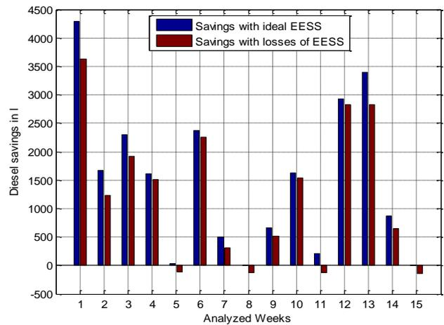
**Figure 9: Calculated diesel savings with a lossfree (ideal) EESS and with the losses of the designed KESS**
