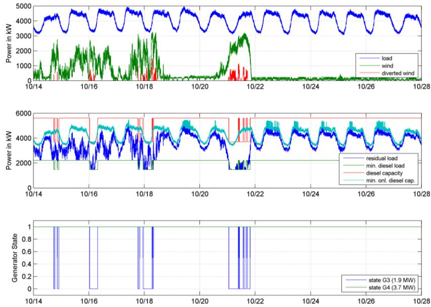
**Figure 7: Load profiles and diesel scheduling with KESS for week 2 and 3**
