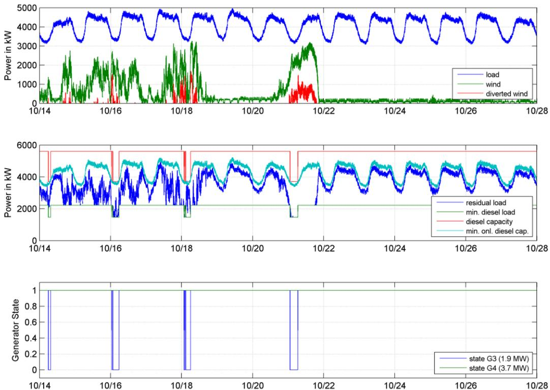
**Figure 1: Load, wind generation and wind diversion (top); residual load, minimal load of diesels, maximum capacity of diesels and minimum online capacity due to SRC rules (middle); states of used diesels (bottom) for week 2 and 3**
