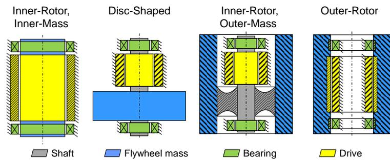
Figure 2: Overview of different flywheel topologies
