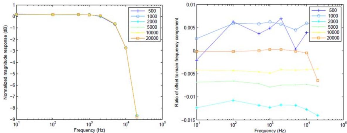
Figure 1: (Left) Magnitude response of the ST100. Different input signal voltages are shown in mV peak to peak. (Right) Offset error of the ST100 as a ratio of the peak to peak input signal voltage. Different signal voltages are shown in mV peak to peak.
