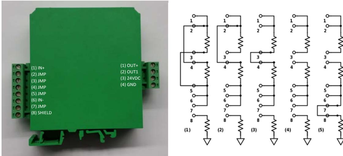
Figure 3: (Left) Input and output connectors. (Right) Wiring of input jumpers for (1) 50 Ω, (2) 100 Ω, (3) 200 Ω and (4) 1 GΩ input impedance. Jumper (5) is wired to ground the negative input when there is no shield on the input line.
