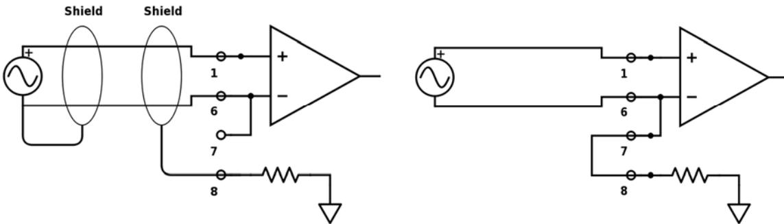
Figure 4: (Left) Wiring of sensor to Shield input with a shielded cable. (Right) Wiring of sensor to Shield input without a shielded cable.
