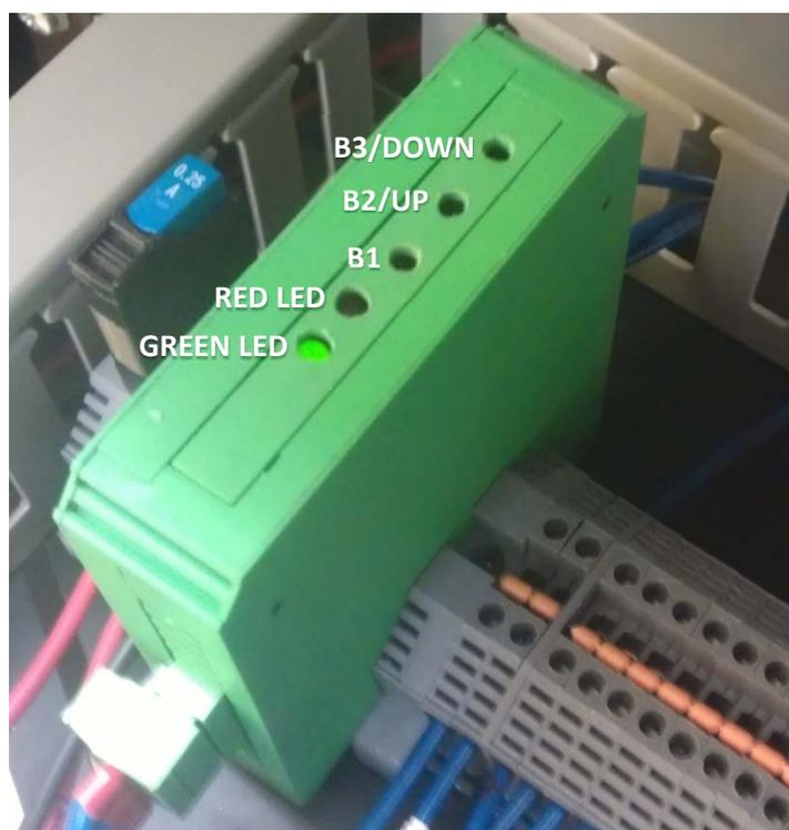
Figure 2: Button and LED locations on the ST100.
