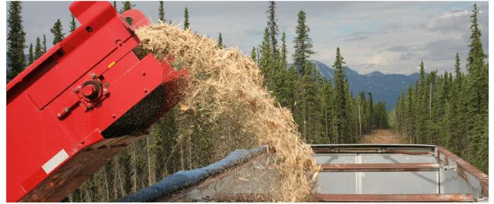
Producing biomass fuel for a wood chip boiler that provides heat and power to the school in Tok, Alaska. Photo by Amanda Byrd/ACEP.
