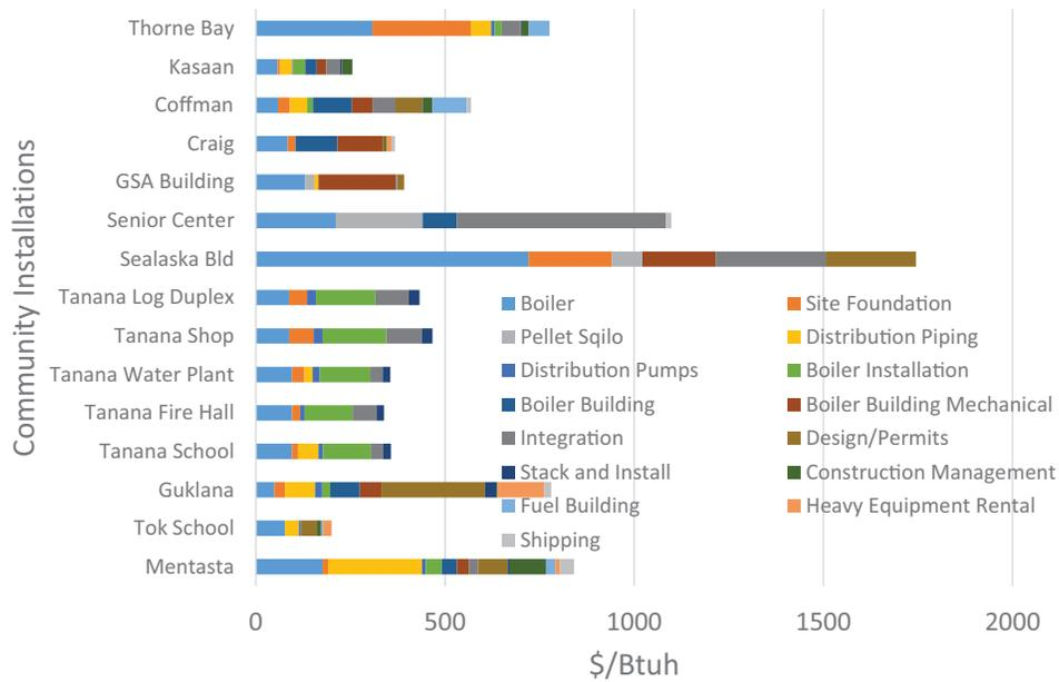
FIG. 5. Installed biomass technology costs by major components (\$/MBtuh).
