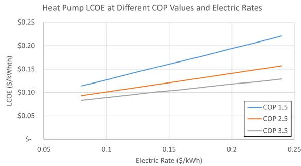
FIG. 4. Heat pump LCOE is plotted at different electric rates and different COP values using a constant set of assumed capital and O&M costs.
