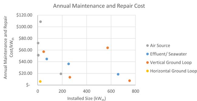
FIG. 2. Maintenance and repair costs per kW<sub>th</sub> along with the system installation size are shown for 14 heat pumps around Alaska. These cost figures include the estimated cost of eventual replacement or refurbishment of the system; the approximate cost of system replacement in 20–25 years. These cost figures do not include the electricity needed to run the systems.
