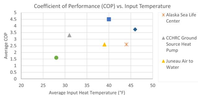
FIG. 3. Average coefficient of performance is plotted according to input temperatures for a variety of heat pumps in Alaska. Warmer input temperatures lead to higher coefficients of performance.
