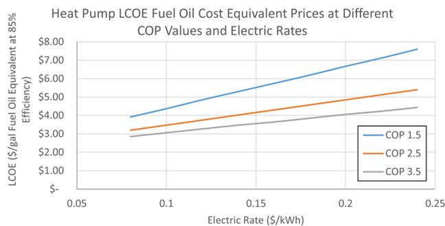
FIG. 5. This graph uses the same input data as Fig. 4. However, LCOE is shown as the equivalent cost of fuel oil when consumed in an 85% efficient boiler.
