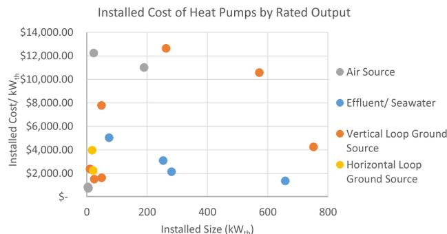
FIG. 1. The installed cost per  $\text{kW}_{\text{th}}$  (thermal) of rated output is compared with the rated output of 17 heat pumps of varying sizes and designs around Alaska.
