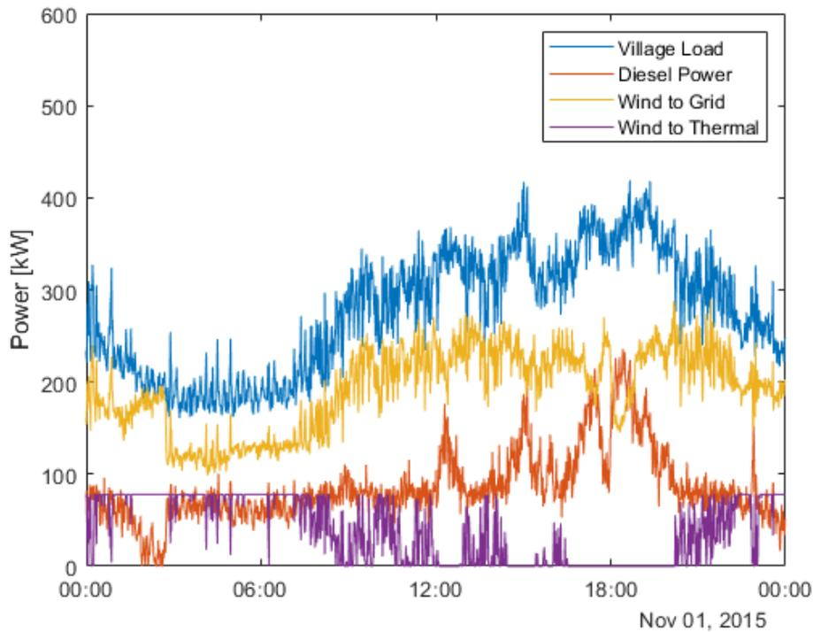
Figure 8. Power data on day of highest wind to heat output.
