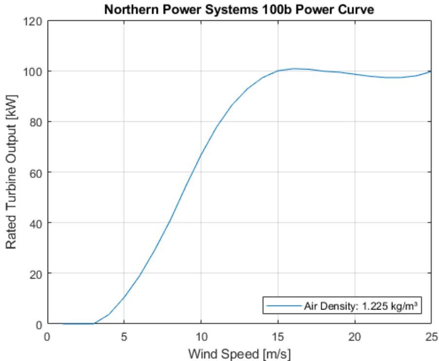
Figure 1. NPS 100b wind turbine power curve
