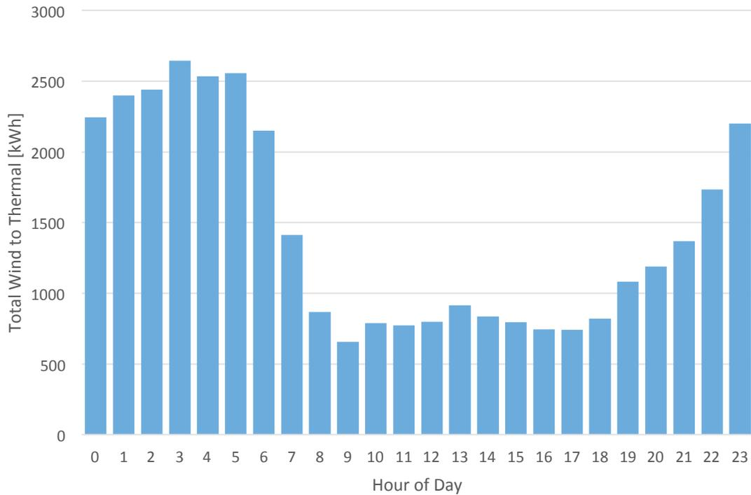
Figure 9. Wind to thermal load by hour of day. Entire dataset.
