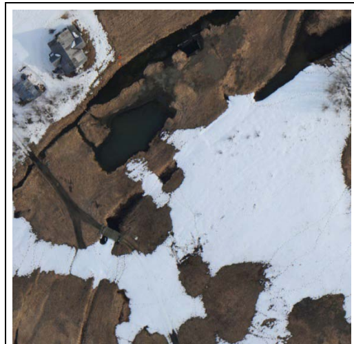
Figure 1. Aerial photograph of Pilgrim Hot Springs, Alaska: geothermally-heated ground is observed as areas of anomalous snow-free conditions in this wintertime image.
